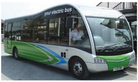
Size of batteries in this application is important: to provide a range of 250 km (~150 miles) implies a battery mass of well over 2 tonnes – equivalent to the weight of some 30 passengers
